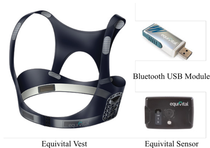
Figure 5.3: Equivital vest and sensor for physiological data measurement
